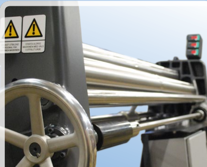
Cone bending equipment, includes diagonal setting of bending roll, trailing shoe and handwheel with dial register
